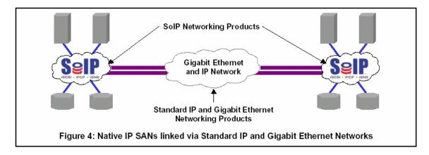
With a native IP SAN solution in place, IT managers can now rapidly deploy applications such as remote backup, mirroring and disaster recovery. The ability to develop highly scalable storage configurations is added through the reach and ubiquity of IP and Ethernet. And storage can be easily consolidated across hosts with an SoIP storage network.
